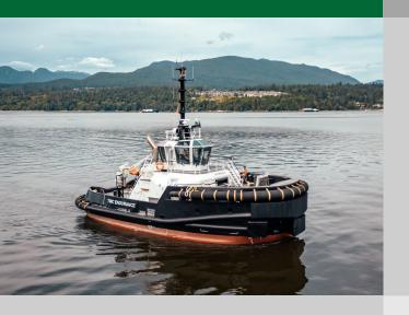
The compact, multi-purpose ASD Tug 2312 delivers a powerful 70 tonnes of bollard pull while the patented Twin Fin skeg plus twin Azimuth thrusters ensure excellent maneuverability. An obstacle-free working deck ensures a safe working environment for the six crew members, as does the powerful covered winch which handles both forward and aft operations.
