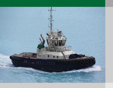
The compact, multi-purpose TWC Artemis is powered by twin 3512C Caterpillar diesels developing 3,000bkW (4,023 bhp) driving twin Rolls-Royce US205 azimuth thrusters and producing a bollard pull of 48.7 tonnes and speed 12.4 knots.
