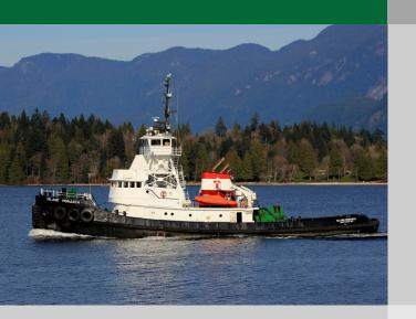
A proven offshore tug of 3000 horsepower, the *Island Monarch* is primarily engaged in pushing and towing of Tidewater Canada's large oil barge fleet.
