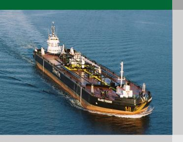
The *Island Trader* is a double hulled, IMO compliant, Class A OPA 90 oil tank barge having an aggregate capacity of 65,000 barrels at 90% carried in twelve separate cargo tanks.
