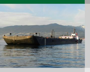
A double-hulled, IMO compliant, OPA 90 oil tank barge. Designed primarily for pushing, the *ITB Vancouver* is equipped with a powerful omni-directional bow thruster for aiding in docking and maneuvering.
