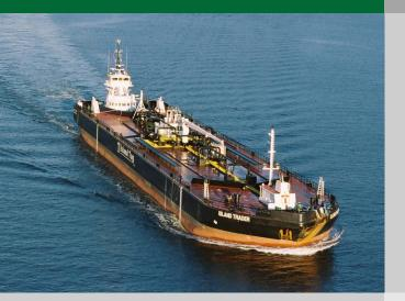
The *Island Trader* is a double hulled, IMO compliant, Class A OPA 90 oil tank barge having an aggregate capacity of 65,000 barrels at 90% carried in twelve separate cargo tanks.
