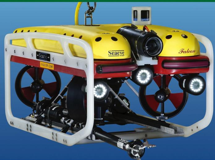
A compact lightweight and versatile Remotely Operated Vehicle (ROV) with a depth rating of 300 metres. The Falcon SeaEye is rapidly deployed on almost any vessel or from shore.
