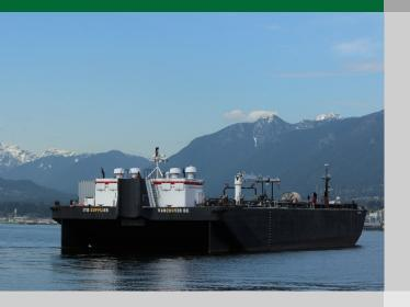
A double-hulled oil tank barge capable of delivering a variety of products quickly and efficiently utilizing three segregated cargo systems.
